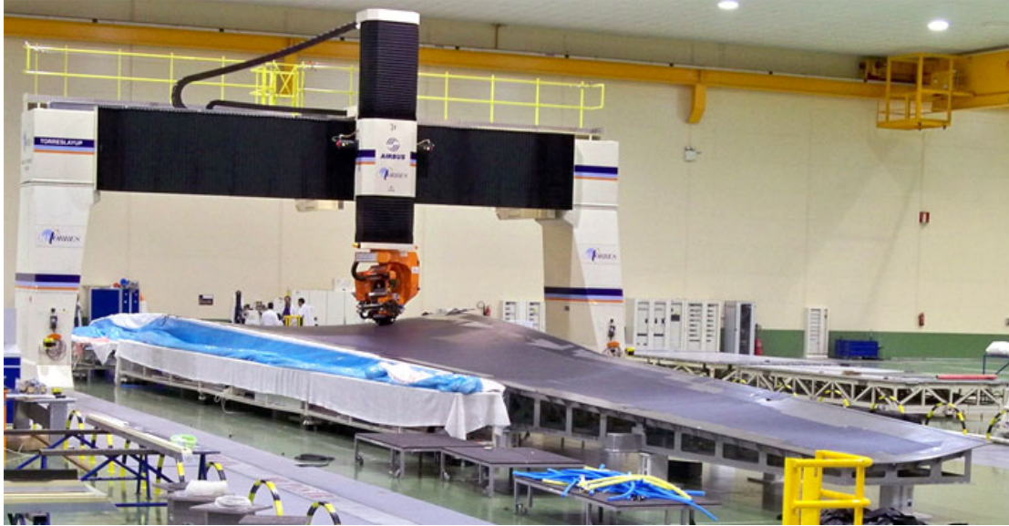
Figure 2. MTorres overhead gantry ATL machine
